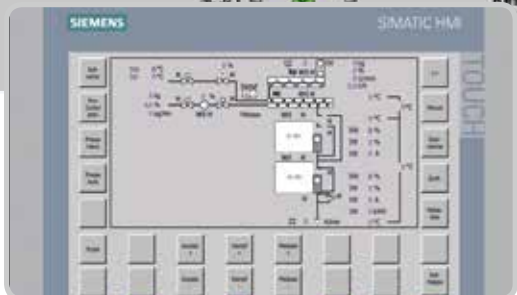
Control of all relevant press parameters with automatic check of flow rates and conveying paths
